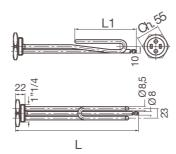
Volt: 220 single-phase, Watt: from 1000 to 3000 (see table) Threaded connection M 1"1/4 GAS - ISO 228/1, Brass CW617N, copper resistance pipe: 8.5 mm, electric connection: Faston, surface charging field: On request with thermostat probe door: L = 275 mm copper, bottom of scale 70-80°C single and double safety device in complance with Standard EN 60730-l
