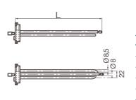
Volt: 220 single-phase, Watt: from 1000 to 3000 (see table) Threaded – Flange ø 48, Flange: Brass CW 61 7N, copper resistance pipe: 8.5 mm, electric connection: Faston, surface charging field: On request with thermostat probe door: L = 275 mm copper, bottom of scale 70-80°C single and double safety device in compliance with Standard EN 607304 (with other values on request) On request with magnesium anode socket
