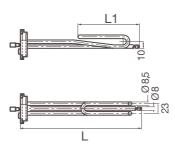
Volt: 22O single phase, Watt: from 1000 to 3000 (see table) Threaded – Flange ø 48, Flange: Brass CW617N, copper resistance pipe: 8.5 mm, electric connection: Faston, surface charging field: On request with thermostat probe door: L = 275 mm copper, bottom of scale 70-80°C single and double safety device in compliance with Standard EN 60730-I (with other values on request) On request with magnesium anode socket
