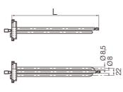
Volt: 22O single phase, Watt: from 1000 to 3000 (see table) Threaded – Flange ø 48, Flange: Brass CW 617N, copper resistance pipe: 8.5 mm, electric connection: Faston, surface charging field: On request with thermostat probe door: L = 275 mm copper, bottom of scale 70-80°C single and double safety device in compliance with Standard EN 60730-I (with other values on request) On request with magnesium anode socket
