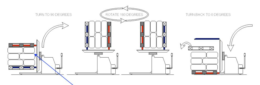
!!! Always keep some space between the bags and the backplates so the bags don't come between the slide bars. Pressure on bags is required!!!
